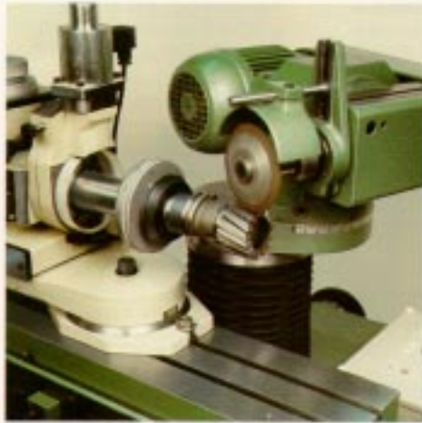
Grind the radial rake angle
