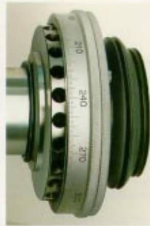
4 24 position indexing plate standard (optional to 38) with 360° adjustable calibrating scale
