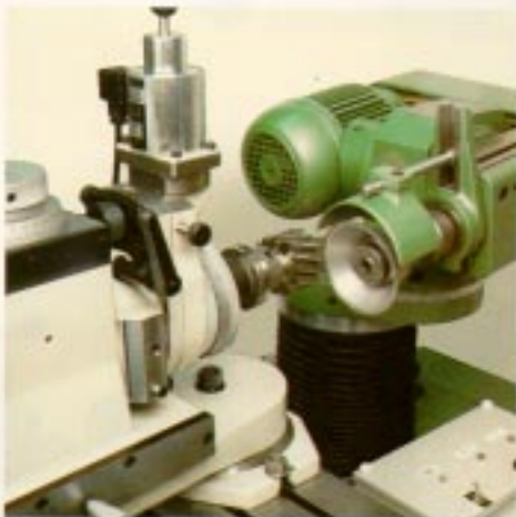
Grind the clearance angles on the end
