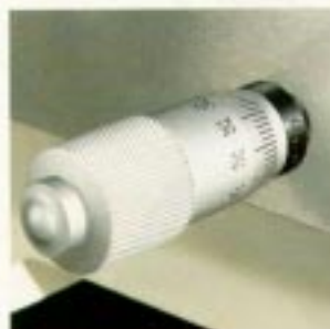
7 Cross slide with micrometer for precise sizing of tool diameter
