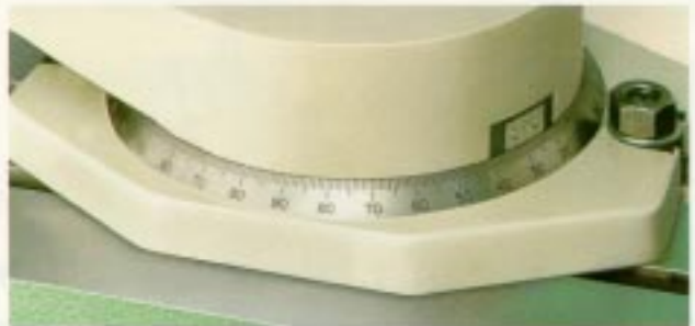
5 Rotating base plate to adjust for grinding position
