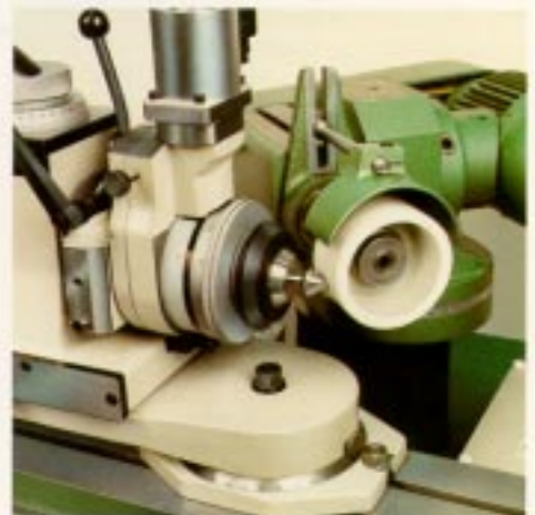
Grind an axial relief angle
