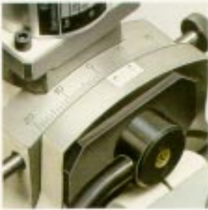
2 Radial infeed with micro adjustment \pm 20^\circ , independent of spiral setting
