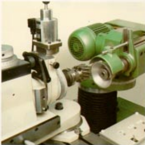
Grind the clearance angles on the end
