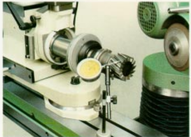
Dial Indicator to set up helix
