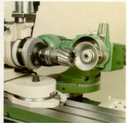
Grind the clearance angles
