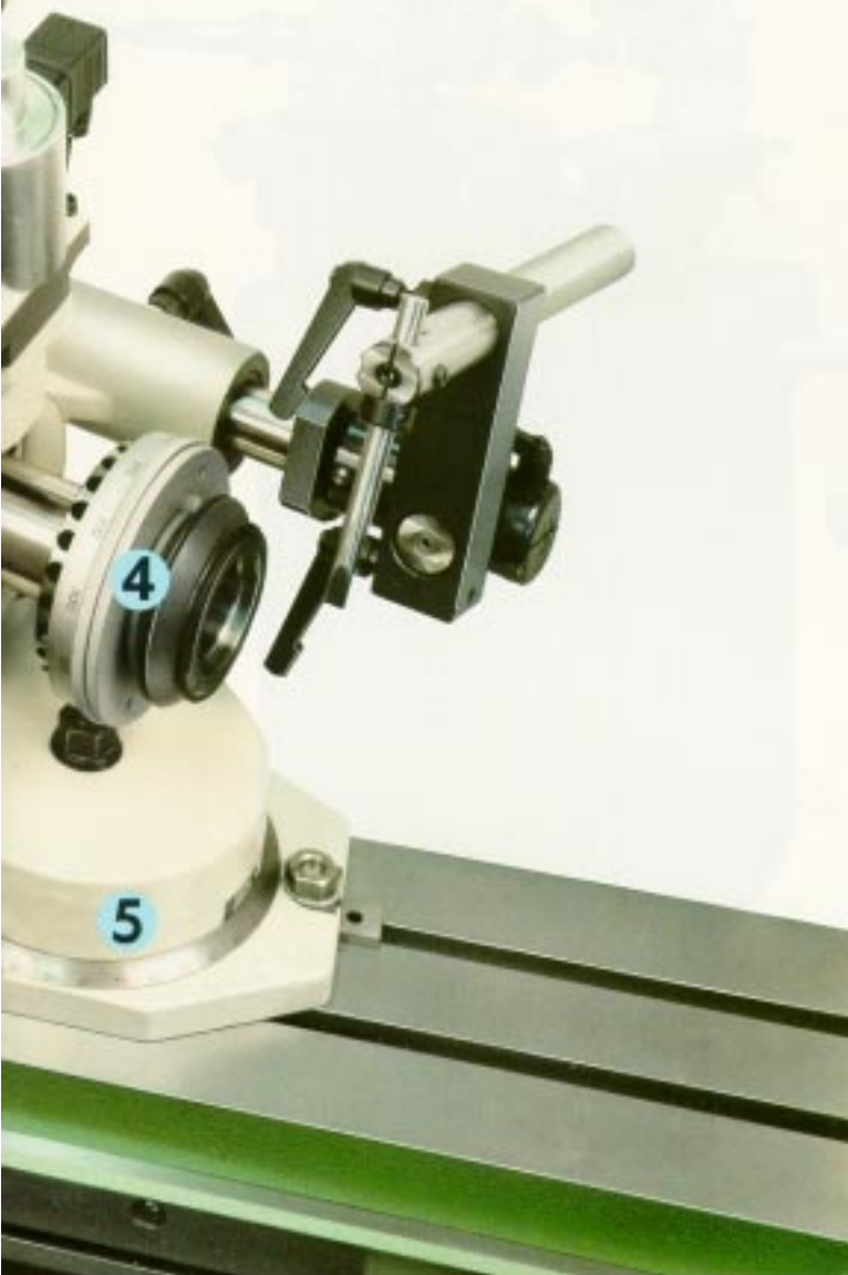
5 Rotating base plate to adjust for grinding position
